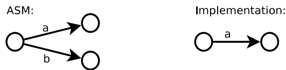
Figure 8: The implementation does not conform to the ASM, because it does not contain every trace of it.
